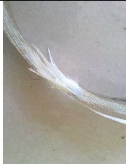
Axial Separation of Advancing Mandrel Pipe in Field (Single line failure due to poor axial strength)
