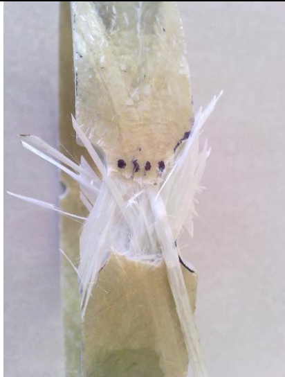
Typical Breaking mode of Helical Wound Pipe During Tensile Testing (Helical fibers does not allow a single line failure)
