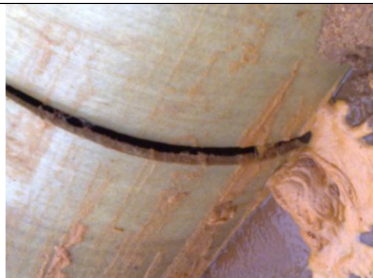
Axial Separation of Advancing Mandrel Pipe in Field (Single line failure due to poor axial strength)
