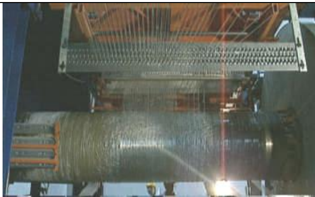
Advancing Mandrel Process with 90° hoop windings
