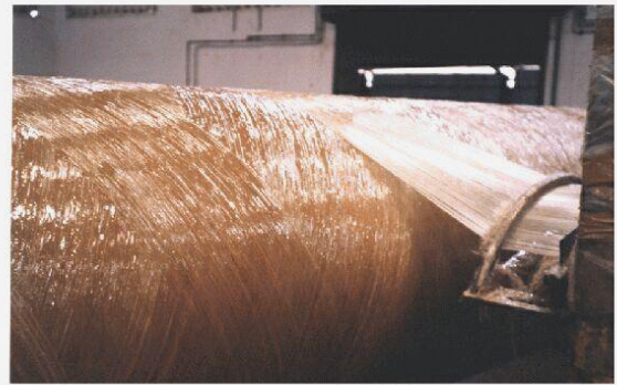
Helical winding Pattern & Interweaving
