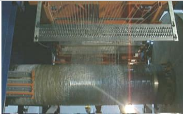
Advancing Mandrel Process with 90° hoop windings
